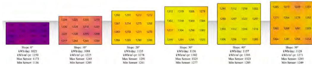
Fig. 11. Annual solar radiation received in same area panels with different slopes.
