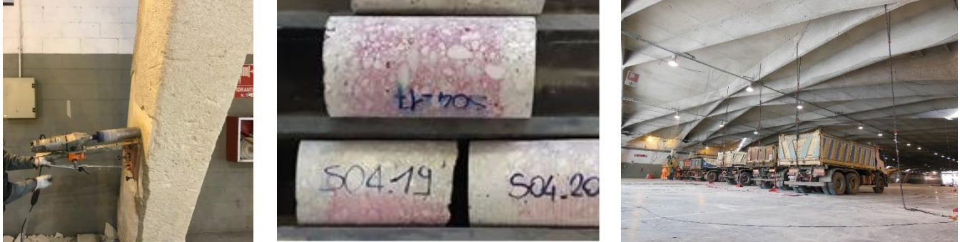
Figure 7 Pavilion V: Extraction of a concrete sample from a longer strut beam (left); carbonation tests on the samples of the ribs (center); view of the static tests with trucks connected to the ribs through jacks (right) [34].
