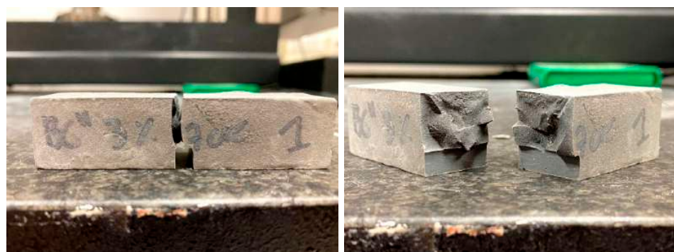
Figure 10. Pseudo-linear crack path and rough fracture surface. B 3% at 7 days.
