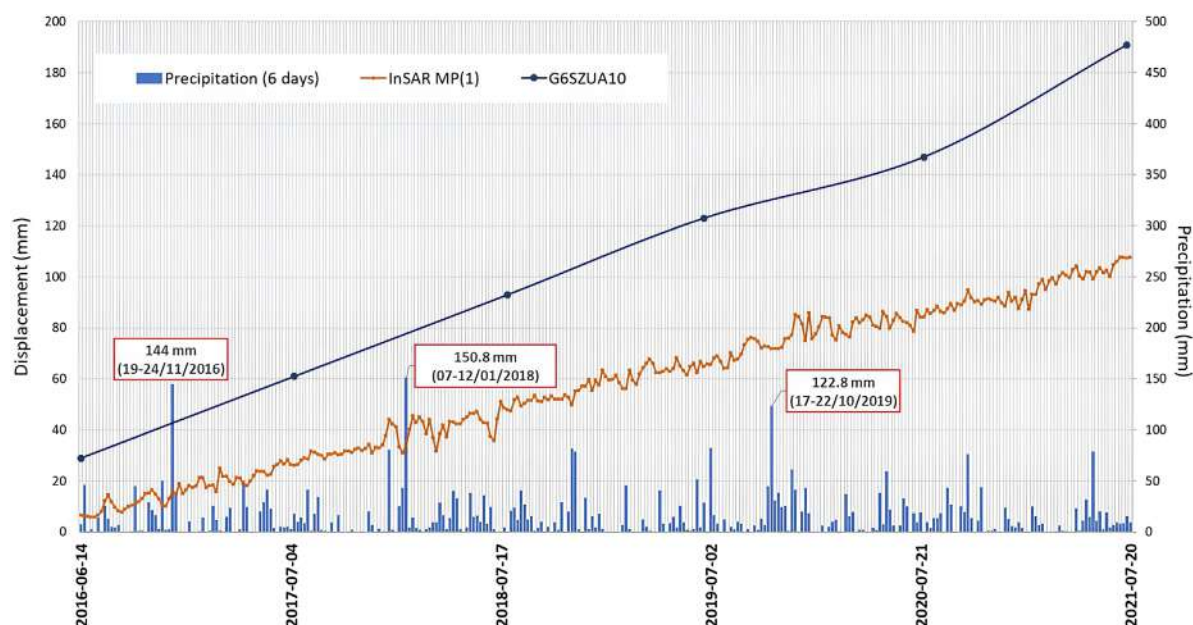
FIGURE 10 Displacements time series at the top of DSGSD in Sauze d'Oulx.
