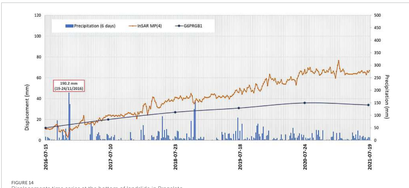
FIGURE 14 Displacements time series at the bottom of landslide in Pragelato.
