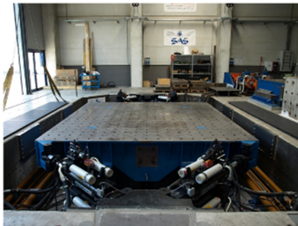
Figure 5: Multi axial shake table - courtesy of EUCENTRE [36]
