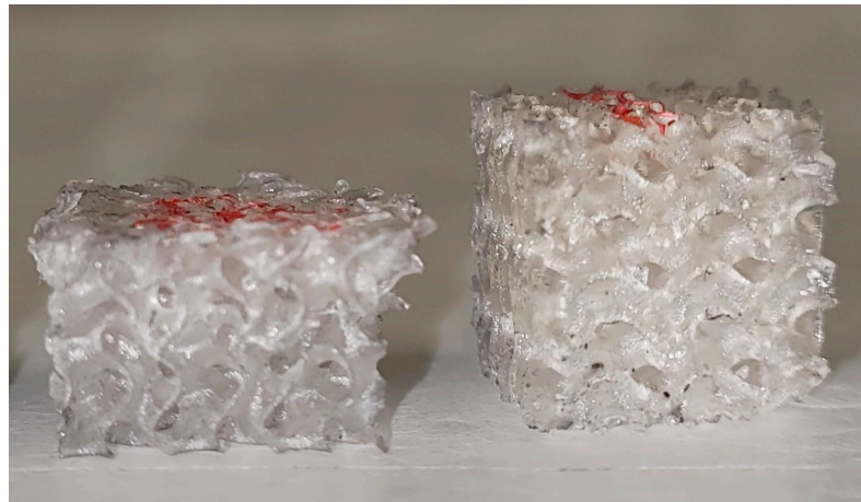
Figure 7. Gyroid-type scaffold before (right) and after the compression test (left).
