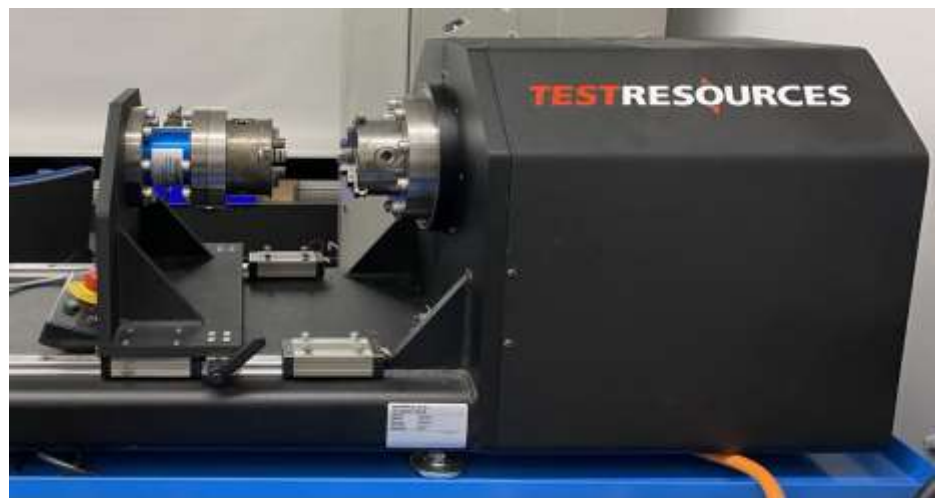
Figure 2. Torsion machine at J-Tech@Polito laboratories.
