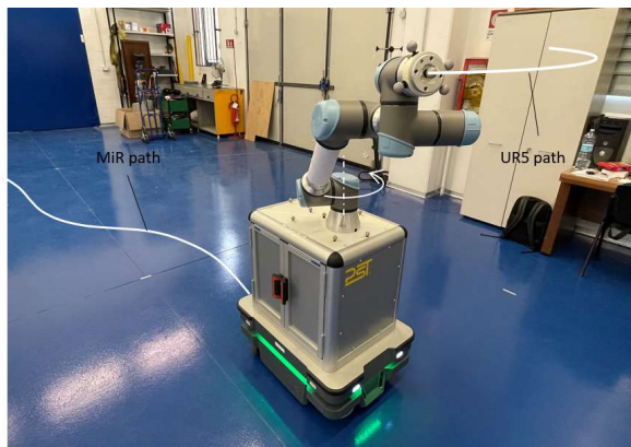
FIGURE 17: COMBINATION OF THE MOTION OF MOBILE ROBOT AND MANIPULATOR
