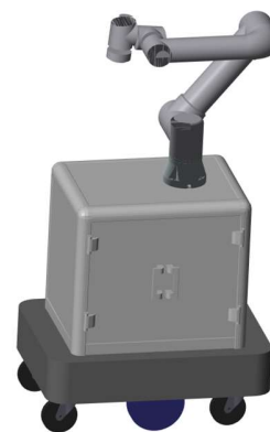
FIGURE 9: GRAPHIC REPRESENTATION OF THE MODEL BY SIMSCAPE MULTIBODY
