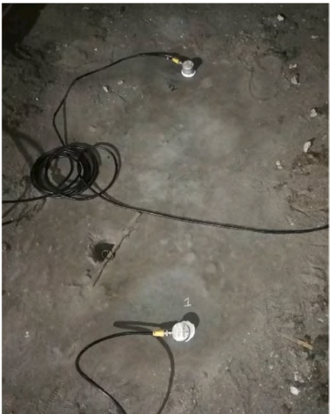
Fig. 7. Two of the eight sensors, positioned on the extrados of the central nave vault.
