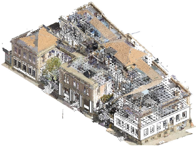
Fig. 11. Point cloud obtained with the 3D laser scanner.
