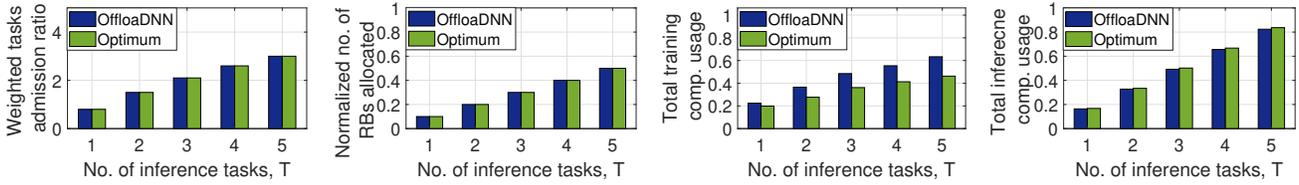
Fig. 8. Small-scale scenario: comparison between OffloadDNN and the optimum as a function of the number of inference tasks  $T$ : (left) average task admission ratio weighted by the tasks’ priority; (center-left) total number of RBs allocated to the tasks’ slices, normalized to the maximum available; (center-right) total compute usage for the training of the active DNNs; (right) total compute usage for the admitted inference tasks, normalized to the maximum available.
