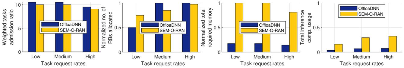
Fig. 10. Large-scale scenario: comparison between OffloadDNN and SEM-O-RAN as the tasks requests rate varies: (left) average task admission ratio weighted by the tasks priority; (center-left) total number of RBs allocated to the tasks slices, normalized to the maximum available; (center-right) total memory utilization for the active DNNs; (right) total compute usage for the admitted inference tasks, normalized to the maximum available.
