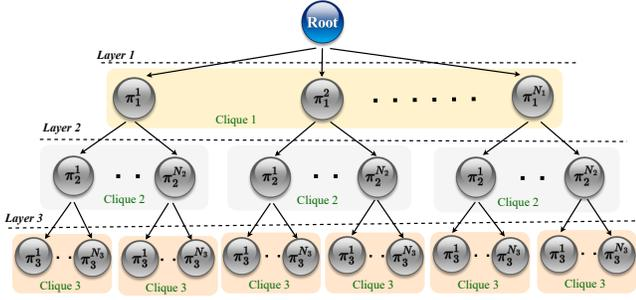
Fig. 5. Hierarchical tree representation for  $T=3$  tasks. Here, task  $\tau=1$  has highest priority with  $N_1$  siblings in clique 1,  $\tau=2$  has second highest priority with  $N_2$  siblings in clique 2, and  $\tau=3$  has third highest priority with  $N_3$  siblings in clique 3. Each vertex  $v_j=\pi_\tau^j$  in the clique at  $t$ -th layer  $t$ .
