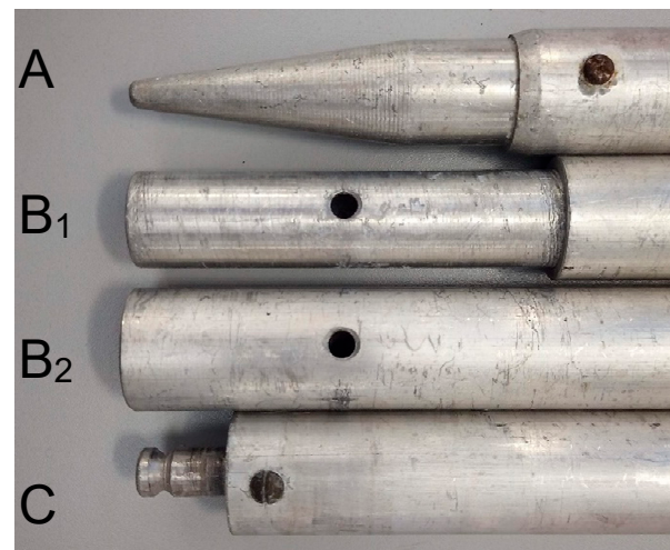
Figure 4. Different details of the aluminum pole: (A) tip; (B 1 ,B 2 ) two ends of the coupling system of the four sections; (C) steel adapter for topographic prism.
