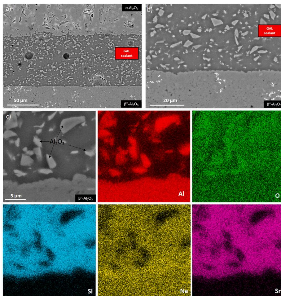
**Fig. 7.** SEM cross-sectional views of (a, b) the  $\alpha$ - $\text{Al}_2\text{O}_3$ /GAL/ $\beta''$ - $\text{Al}_2\text{O}_3$  joined sample obtained after curing at 900 °C for 40 min and (c) EDS elemental maps of the sealing area; the black arrows indicate alumina particles.
