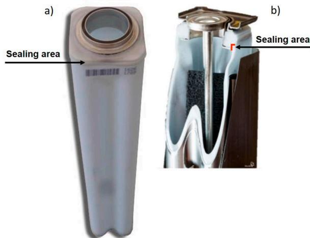
**Fig. 1.** Single solid-electrolyte cell produced by the FZSoNick SA company [4]: (a) front-view and (b) cross-section in which the sealing area between the  $\alpha$ -Al<sub>2</sub>O<sub>3</sub> collar and the  $\beta''$ -Al<sub>2</sub>O<sub>3</sub> solid-electrolyte tube is indicated by the black arrow.
