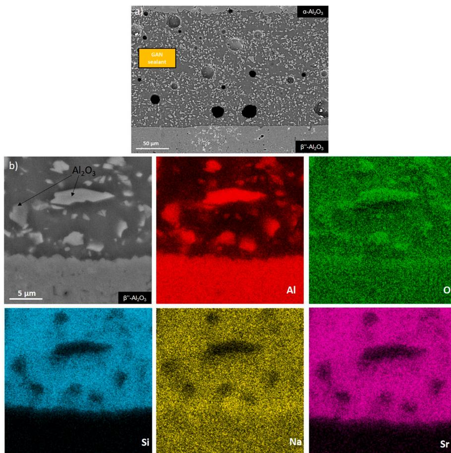
**Fig. 8.** SEM cross-sectional view of (a) the  $\alpha$ - $\text{Al}_2\text{O}_3$ /GAN/ $\beta''$ - $\text{Al}_2\text{O}_3$  joined sample obtained after curing at 900 °C for 40 min and (b) EDS elemental maps of the sealing area; the black arrows indicate alumina particles.
