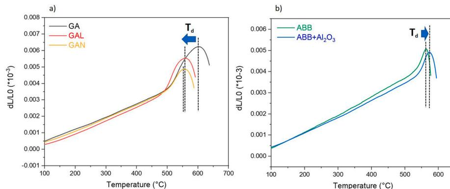
**Fig. 5.** Dilatometry curves of (a) GA, GAL and GAN and (b) ABB, ABB+Al<sub>2</sub>O<sub>3</sub> obtained after sintering at 900 °C for 40 min and 700 °C for 1 h, respectively; all the analyses were carried out with a heating rate of 5 °C/min.
