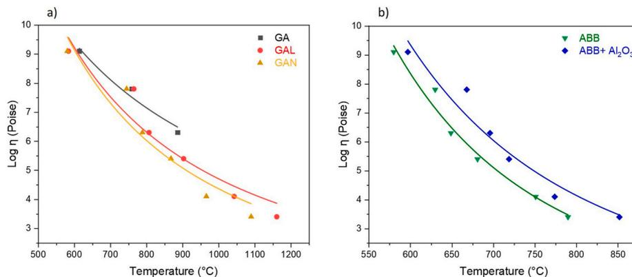
**Fig. 4.** Log η vs Temperature curves for (a) the G018-402-based systems and (b) the ABB-based systems obtained by fitting the characteristic fixed viscosity points and related temperatures [25], calculating.
