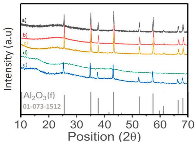
**Fig. 9.** XRD pattern of the following glass sealant candidates: (a) GA, (b) GAL, (c) GAN sintered at 900 °C for 40 min; (d) ABB and (e) ABB+ $\text{Al}_2\text{O}_3$  sintered at 700 °C for 1 h. (f) PDF card (number: 01-073-1512) of  $\text{Al}_2\text{O}_3$ .
