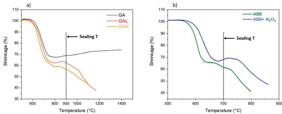
**Fig. 2.** HSM curves of (a) GA, GAL and GAN and (b) ABB, ABB+Al<sub>2</sub>O<sub>3</sub> glass-based sealants; all the analyses were carried out at 5 °C/min heating rate, from room temperature up to the flow temperature detected by the instrument. The black arrow indicates the selected sealing temperature for each glass-based system. ..
