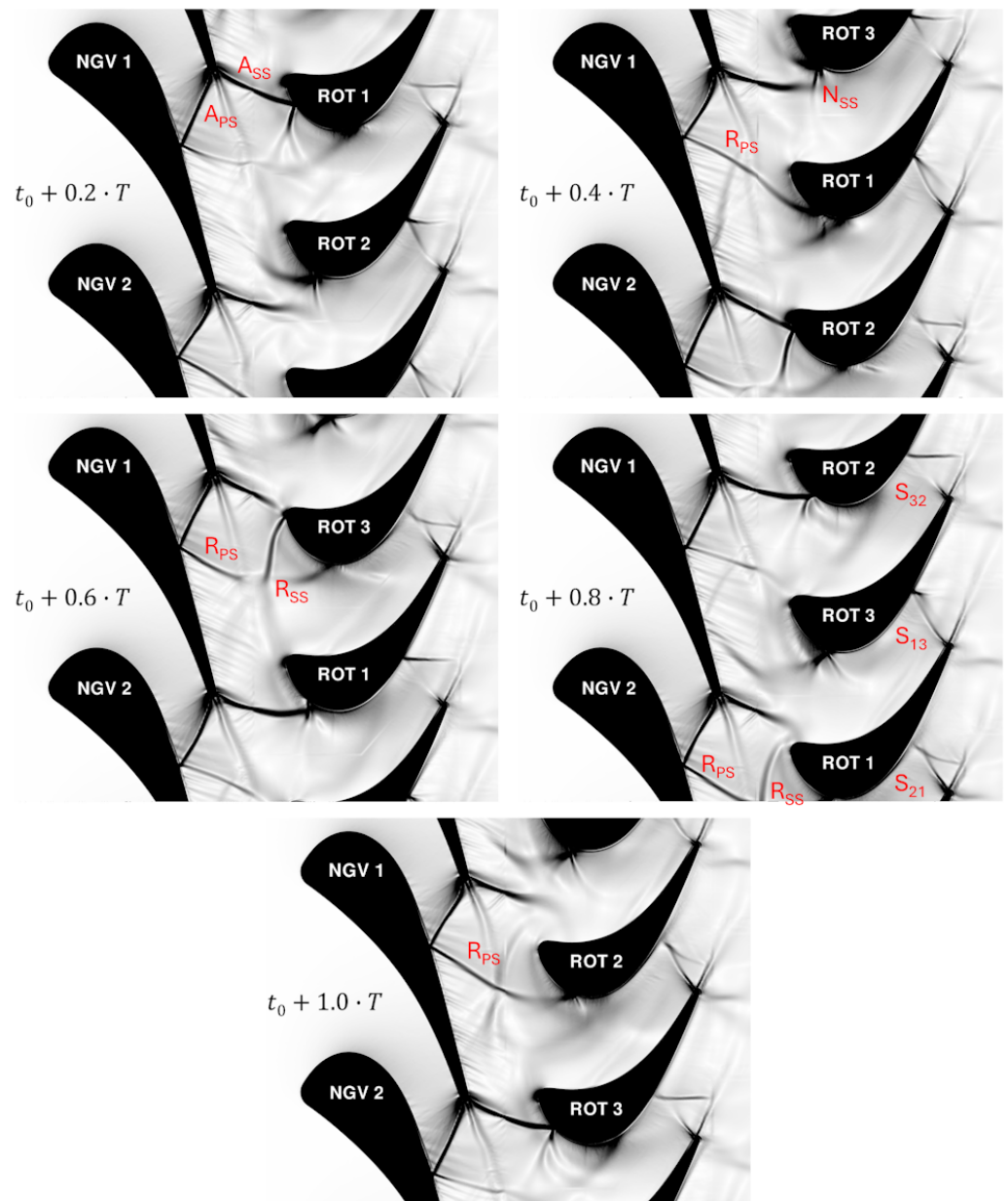
Figure 10. Numerical Schlieren visualization of the shock system occurring in the CT3 high-pressure turbine stage at mid-span (adapted from [123]).
