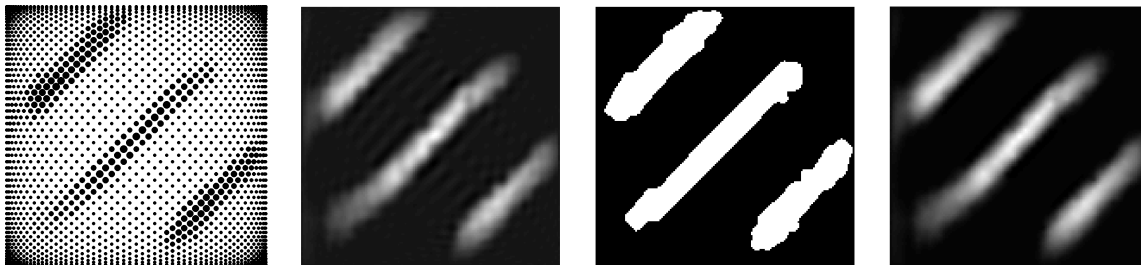
Fig. 7: Comparison of different interpolation methods in MPI. The reconstructed data on the Lissajous nodes \mathbf{LS}_2^{(33,32)} (left) is first interpolated using the polynomial scheme derived in [12] (middle left). Using a scaling function constructed upon a threshold strategy (middle right) the second interpolation is performed by the VSDK scheme (right).
