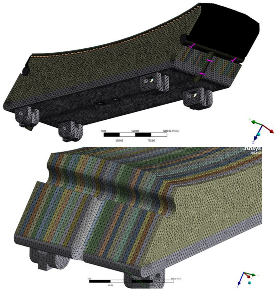
Fig. 34. Overview of developed mesh.
