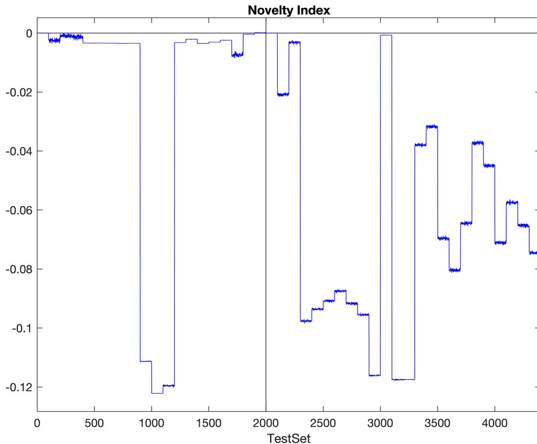
**Figure 5.** Novelty Index NI, for the monitored set M. The feature vectors regard the transmissibilities between two points near the wingtip on the right side. The first 2000 features correspond to the configuration with no winglets. The subsequent ones correspond to the configuration with winglets.
