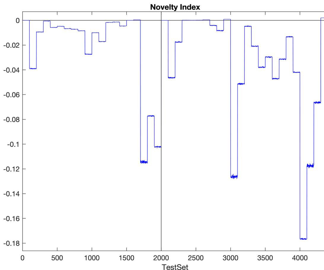
**Figure 4.** Novelty Index NI, for the monitored set M. The feature vectors regard the transmissibilities between two points near the wingtip on the left side. The first 2000 features correspond to the configuration with no winglets. The subsequent ones correspond to the configuration with winglets.
