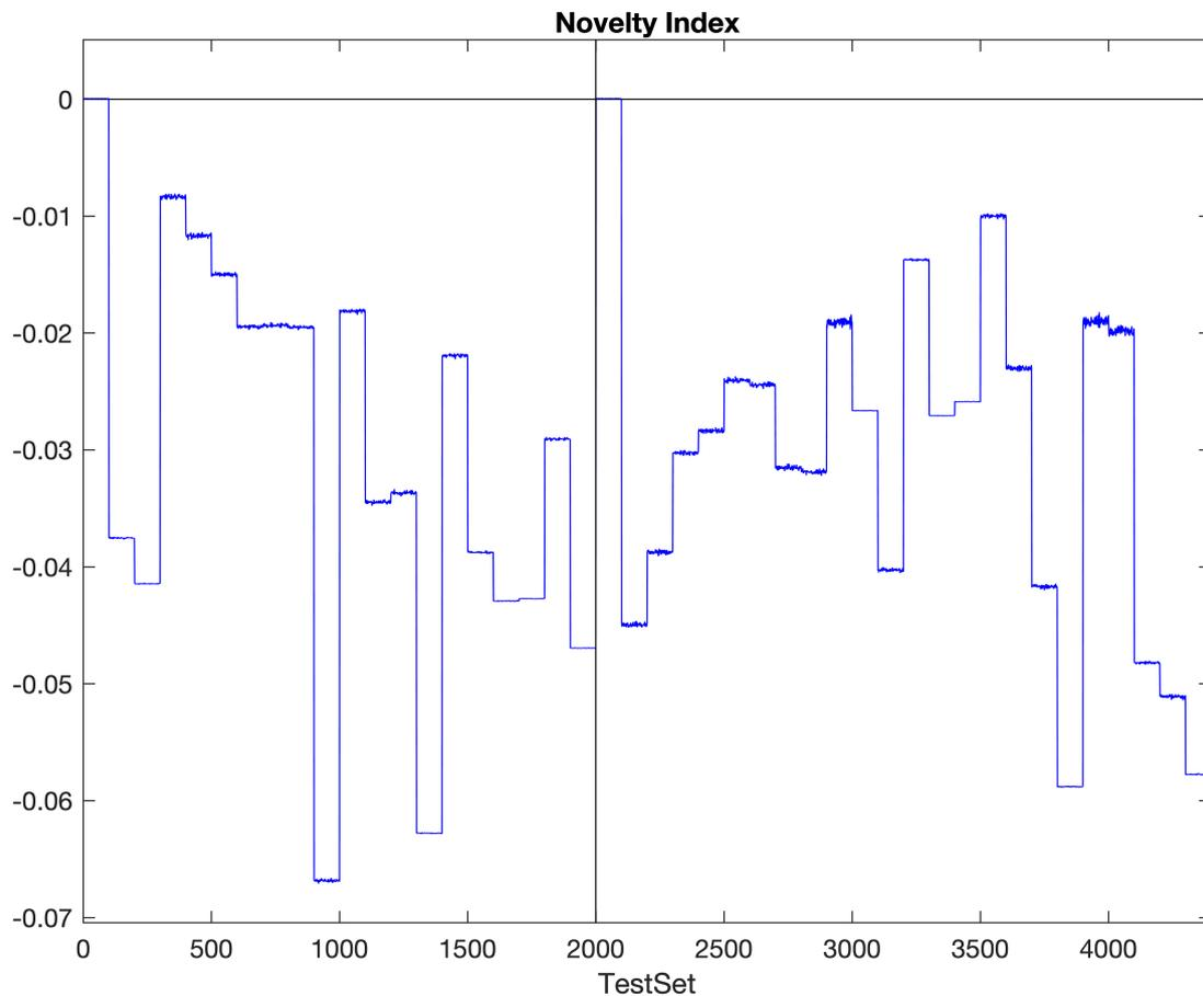
**Figure 3.** Novelty Index NI, for the monitored set M. The feature vectors regard the transmissibilities between the wingtips. The first 2000 features correspond to the configuration with no winglets, the subsequent ones correspond to the configuration with winglets.
