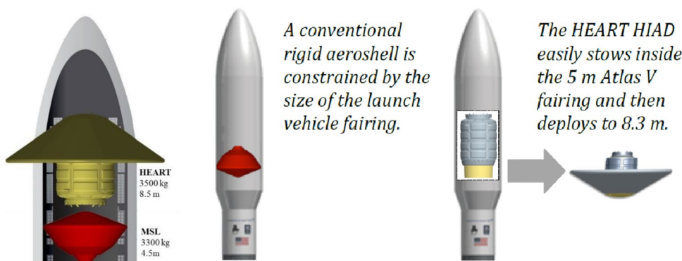
Fig. 1 Rigid heat shield (MSL) and inflatable heat shield concept (HEART, NASA)
