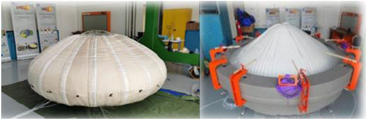
Fig. 20 Static-load testing of the EFESTO inflatable heat shield ground demonstrator
