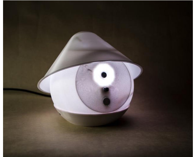
Figure 11 | Shybo robot: a high-fidelity and semi-functioning prototype.
