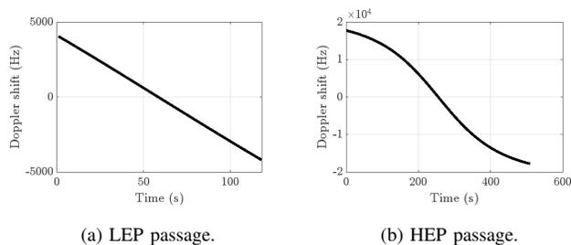
Fig. 6: Doppler shift for different satellite passages.
