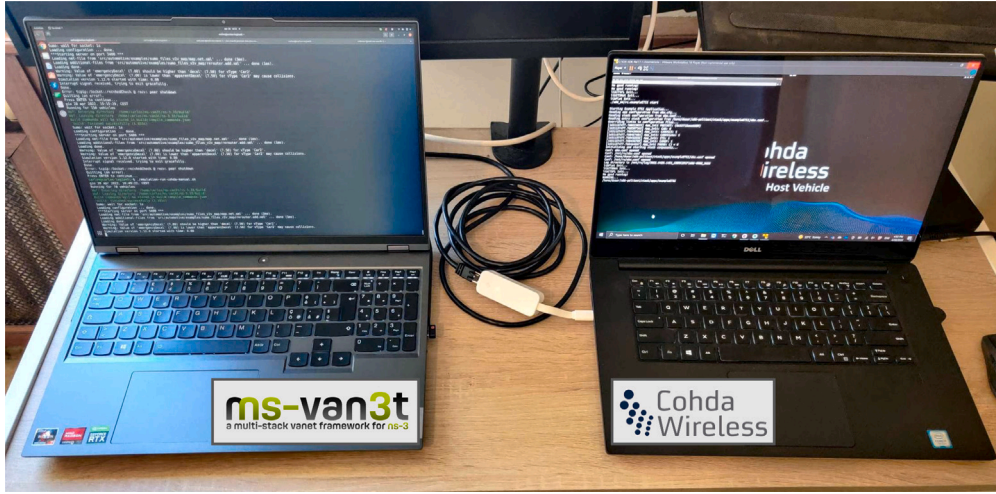
Fig. 10. Laboratory setup for the interoperability tests, performed to validate the emulation feature available in ms-van3t.
