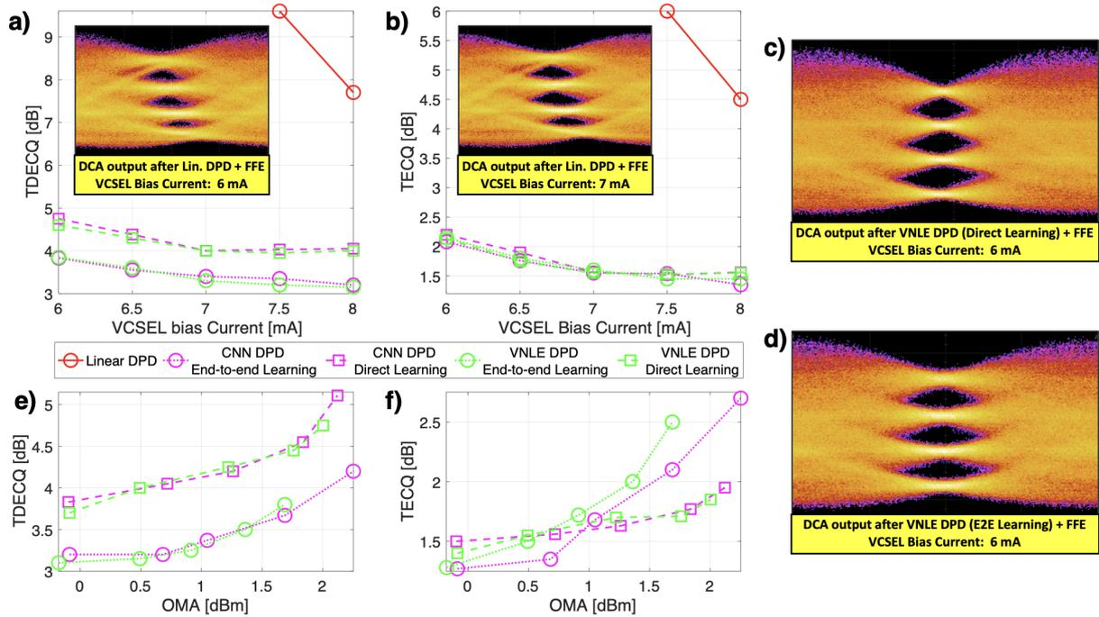
**Fig. 4:** Experimental performance results: (a) TDECQ vs VCSEL bias current (b) TECQ vs VCSEL bias current (e) TDECQ vs VCSEL OMA (f) TECQ vs OMA. Eyediagrams at DCA output for low bias currents showed in (a, inset), (b, inset), (c) and (d)
