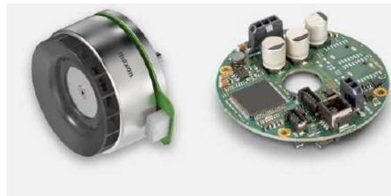
Figure 21. Chosen motor (left) and the inverter (right).
