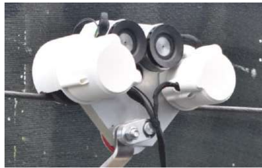
Figure 24. Trolley traction structure with 3D-printed cover.
