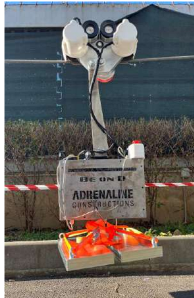
Figure 33. Electric trolley with 55 kg payload.
