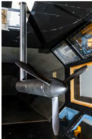
(a) Isolated propeller with three blades installed on a sting
