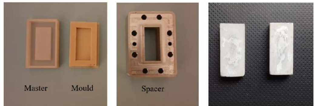
Figure 2. Master and mold for sample preparation. Spacer for WR137 waveguide measurements. Samples of cement-based composites with no fillers.
