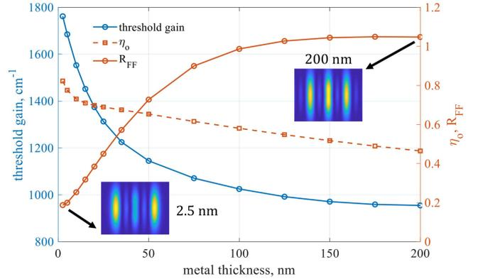
Fig. 7. Impact of the metal thickness on the threshold gain  $G_0^x$ , outcoupling efficiency  $\eta_o$  and FF ratio  $R_{\text{FF}}$  for the design C.
