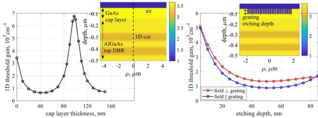
Fig. 5. Left: calculated threshold gain from 1D simulations as a function of the cap layer thickness. The inset represents the refractive index map of the structure, highlighting the 1D cut. Right: calculated threshold gain for the fields parallel and orthogonal to the grating bars with a fixed value of cap layer thickness of 90 nm. The inset shows the investigated sub-wavelength grating.
