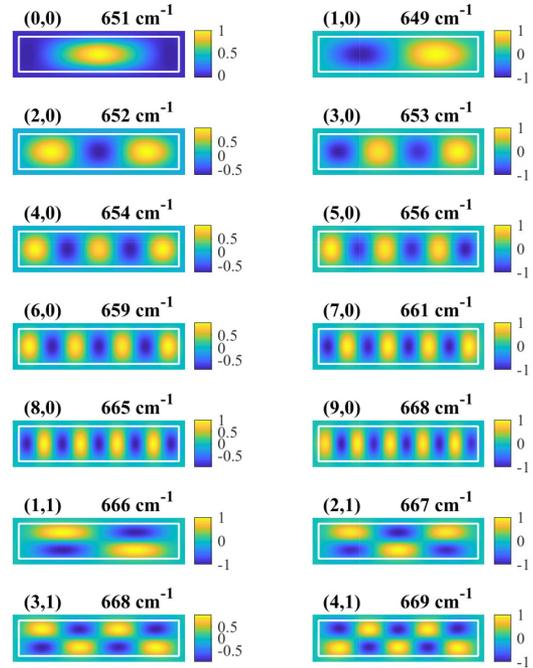
Fig. 2. Calculated mode profiles at the outcoupling facet of a rectangular VCSEL with their corresponding threshold gain. Only  $x$ -polarization is displayed;  $y$ -polarization features exactly the same threshold gain, wavelength and field profile, since in the simulation no intrinsic anisotropy is included. Each mode is indexed by the number of nodes along  $x$  and  $y$ . Emission wavelengths are closely packed: all the modes in the figure lie within a wavelength interval of 0.5 nm.
