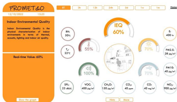
Figure 4. Screenshot of the dashboard. The user can get an indication of the actual IEQ at a glance.
