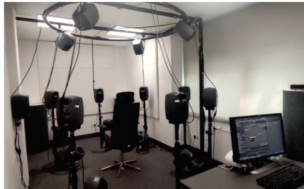
Figure 3. Picture of the Audio Space Lab hosting the designed 3OA sound reproduction system.
