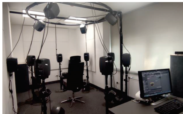
Figure 3. Picture of the Audio Space Lab hosting the designed 3OA sound reproduction system.
