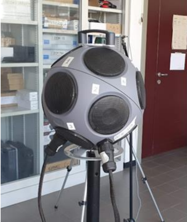
Figure 1. “DodecMIMO” sound source.
