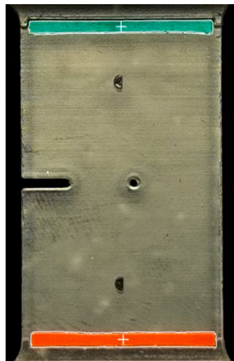
Fig. 9. Video frame of a specimen type A1 with R = 0.5 mm (nominal) showing the digital recognition of the green (upper) and red (lower) optical markers. Each cross represents a marker barycenter.
