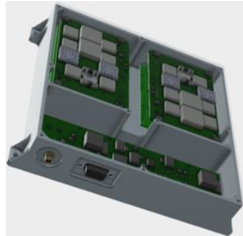
Figure 4: LuGRE QN400-SPACE GNSS Receiver
