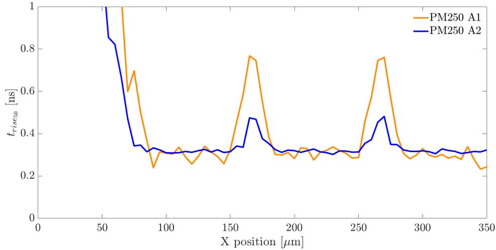
**Figure 10.** Rising edge profiles extracted from a horizontal cut-plane parallel to the x-axis in the rising edge maps.
