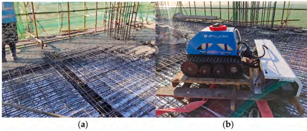
Fig. 14. Field test of concrete curing robot: (a) Engineering appearance of concrete curing site; (b) Concrete curing robot body.
