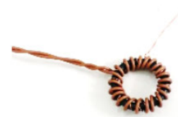
FIGURE 6. FeSi2.9 Toroid: size and shape not fully compliant with the IEC 60404 series standards.
