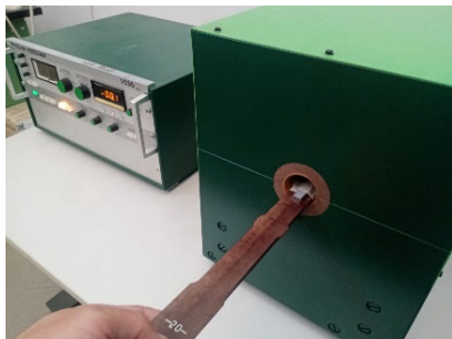
FIGURE 5. Specimen insertion in the coercimeter coil.
