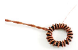
FIGURE 6. FeSi 2.9 Toroid: size and shape not fully compliant with the IEC 60404 series standards.
