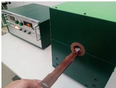
FIGURE 5. Specimen insertion in the coercimeter coil.
