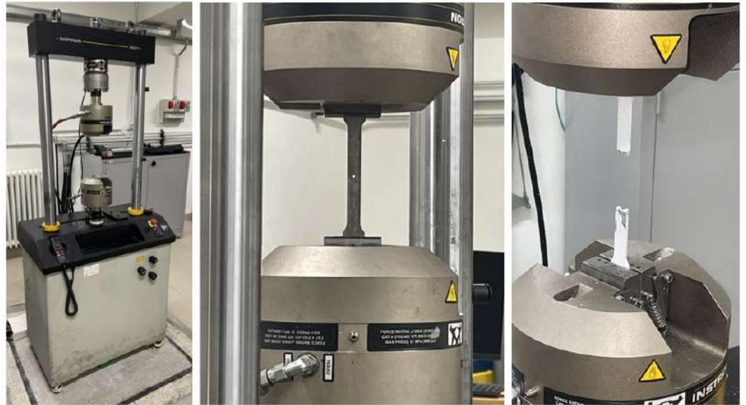
Figure 4. Specimen installed in the fatigue test machine.
