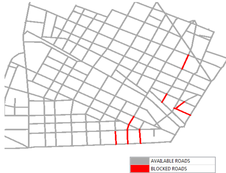
Figure 3. Blocked roads after the seismic event.
