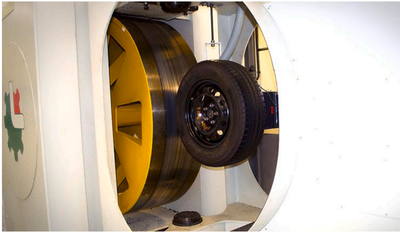
Fig. 15. Leonardo SCRFT test bench.
