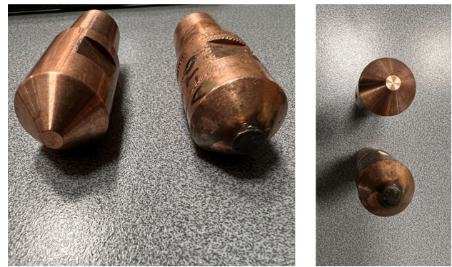
Fig. 7 Example of electrode before and after the experiments
