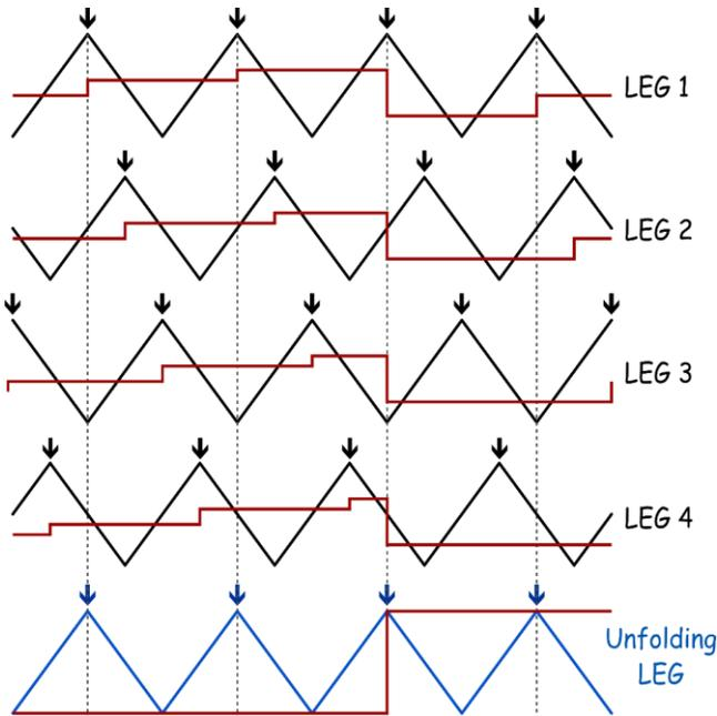
**Fig. 19** Triangular carrier and reference duty cycles of the four switching and unfolding legs. The interrupt service routine and the output duty cycle updates for all the converter legs are performed in correspondence with the green arrow.
