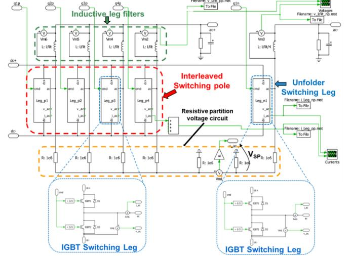
Fig. 9 Block schematic of the single-phase inverter topology with an interleaved switching pole and unfold switching leg used in PLECS® simulation runs.
