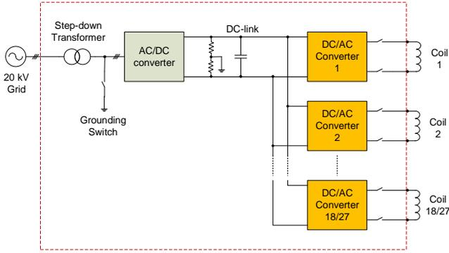
**Fig. 2** Block schematic of the multi-converter power supply for the DTT NAS coils.
