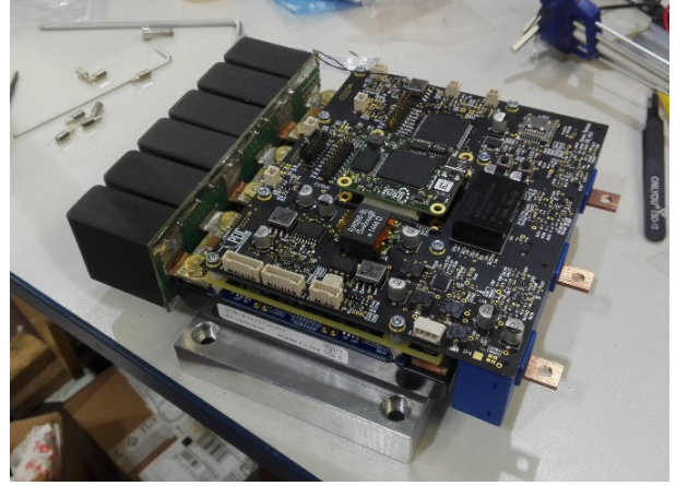
Fig. 1. Prototypal three-phase SiC inverter.
