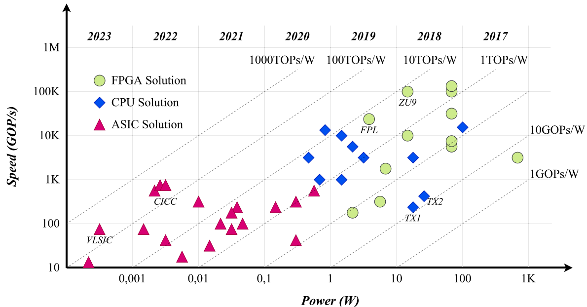
FIGURE 1. A glance at the latest hardware developed for TinyML reveals a notable trend: recent advances focus on minimizing power consumption. This implies that the primary emphasis is enabling ML to run on devices with limited resources.
