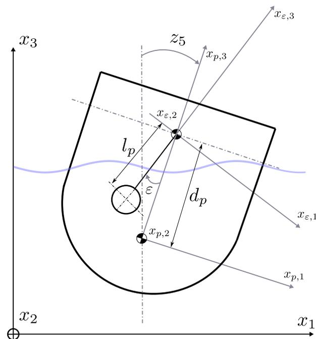
Figure 1. The PeWEC working principle in a schematic two-dimensional fashion.
