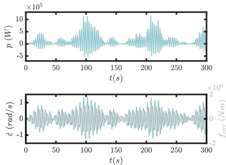
Figure 12. Device response when subject to a panchromatic wave condition, with the instantaneous power displayed at the top, and the PTO velocity  $\dot{\epsilon}$  (in blue) and control force  $f_{ctrl}$  (in grey) at the bottom. The wave spectrum is characterised by the following properties:  $T_p = 6.5$  s,  $H_s = 2.375$  m, and  $dir = 0$  deg.
