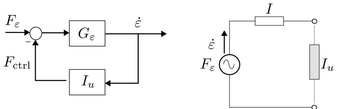
Figure 5. Impedance-matching principle: equivalent electrical circuit representation.
