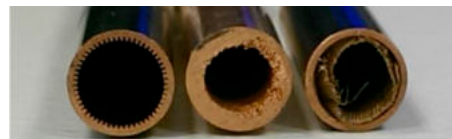
Figure 15. Axial groove, mesh, and sintered cross-section [56].
