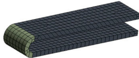
Figure 7. Crotch 3D mesh.
