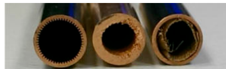
Figure 15. Axial groove, mesh, and sintered cross-section [56].
