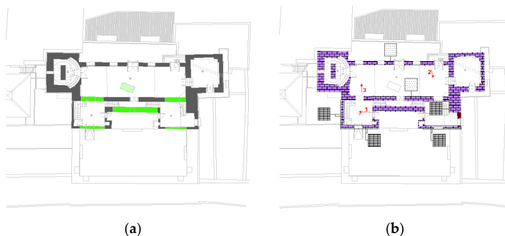
Figure 22. Identification of the structure of the Tower on level L (height 37.70 m): (a) hypothesized vertical load-bearing structure; (b) hypothesized materials.
