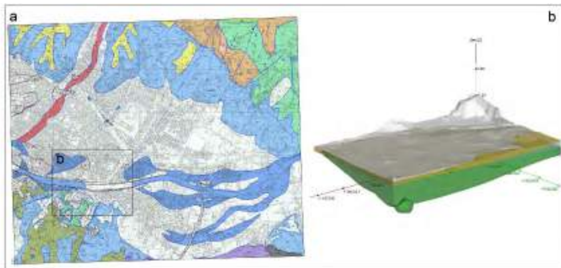
Figure 1. a) The Florence urban settlement as depicted in the 1:10.000 Tuscany geological map (CARG 1:10.000 section n. 275040). The city of Florence well fits with the hypothetical urban settlement proposed in the Scenario n. 5. b) An example of 3D geo-model produced for a portion of the Florence urban area. The 3D model highlights the subsurface stratigraphy and structural setting.
