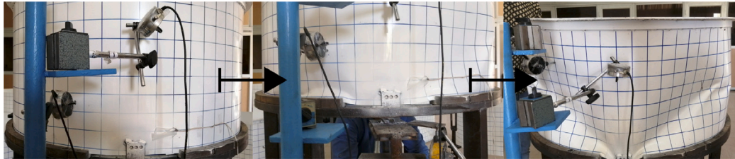
Fig. 4. Progressive buckling of a thin-walled steel tank subjected to local support settlement. Photos by courtesy of H. Naseri (Urmia University).
