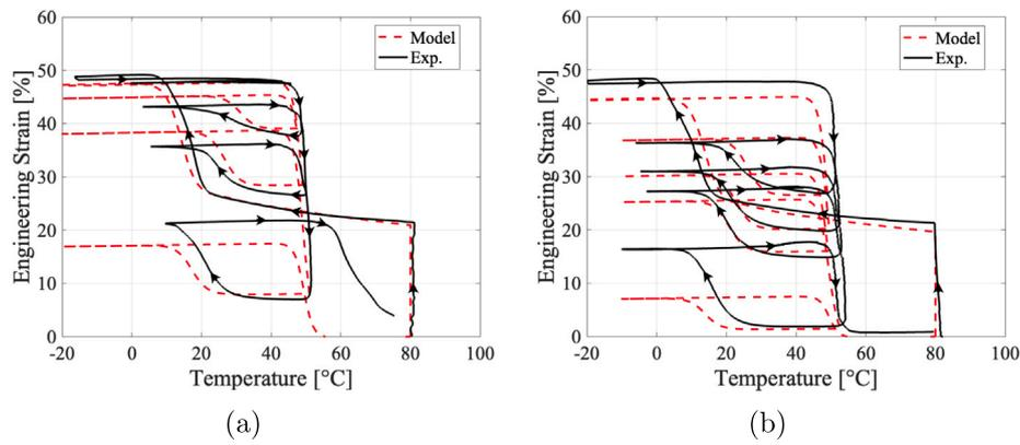
Fig. 18. Engineering strain vs temperature experimental (black-solid) and model (red-dashed) curves demonstrating the effect of  $T_{act}$  on the stress-free two-way SME. (For interpretation of the references to color in this figure legend, the reader is referred to the web version of this article.)
