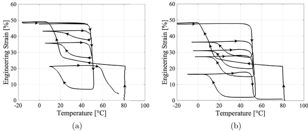
Fig. 8. Strain vs temperature curve demonstrating the effect of  $T_{act}$  on the stress-free two-way SME carried out on two specimens of the same material. Arrows indicate the direction in which steps are applied.
