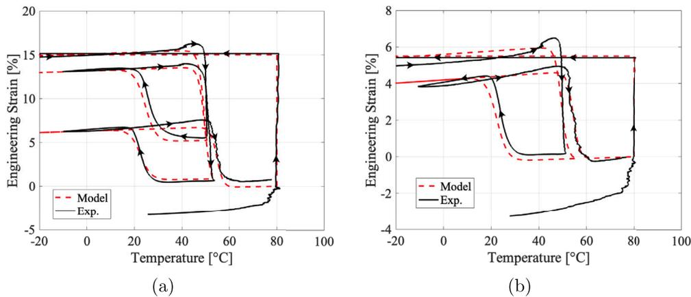
Fig. 19. Engineering strain vs temperature experimental (black-solid) and model (red-dashed) curves demonstrating the effect of  $T_{act}$  on the stress-free two-way SME for an applied tensile pre-strain of (a) 15%, (b) 5.5%. (For interpretation of the references to color in this figure legend, the reader is referred to the web version of this article.)
