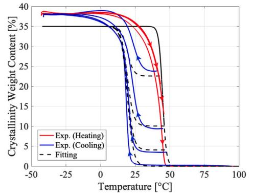
Fig. 14. Model validation on cyclic crystalline-temperature curves.
