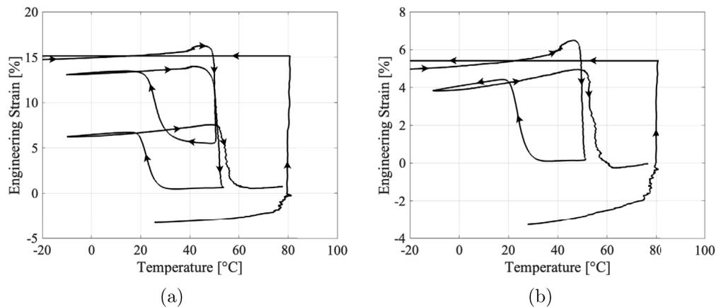
Fig. 9. Strain vs temperature curve demonstrating the effect of  $T_{act}$  on the stress-free two-way SME. Two pre-strains equal to (a) 15% and (b) 5.5% were considered. Arrows indicate the direction in which steps are applied.
